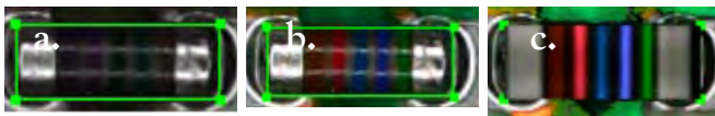
Figure 4a. Greyscale melf resistor values. 4b. 24-bit colour. 4c. 24-bit colour with synthetic imaging.
